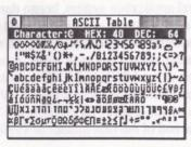
This displays the full complement of Atari ASCII characters and allows you to insert these into the text using the macro processor. It gives you the decimal and hexadecimal value of the key as well.
